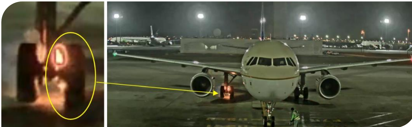
Figure 4: A320-211 fire on the right main landing gear
