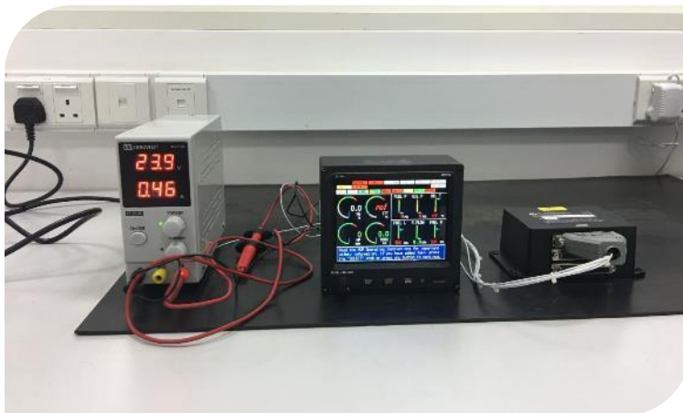
Figure 7: MVP-50T connections for download
