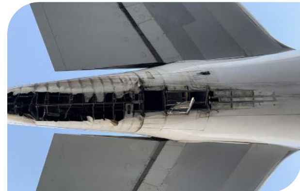
Figure 2: Tail strike damage
